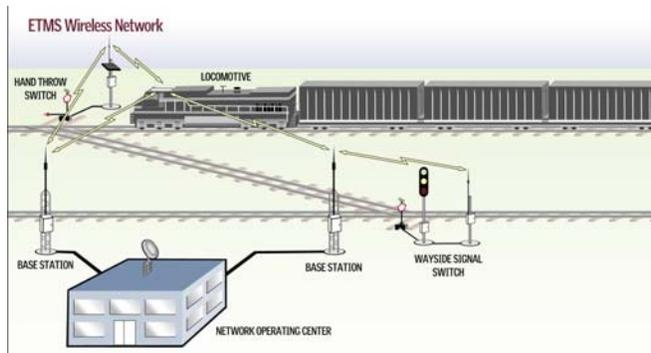
**The Positive Train Control (PTC) system utilizes a wireless network to communicate to the primary system components.**
